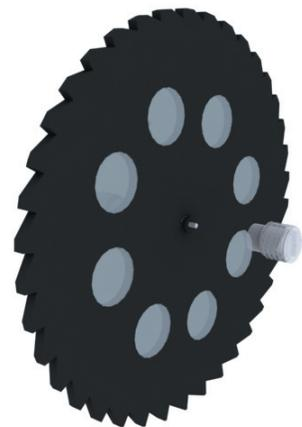
Figure 2: Wheel and bearing assembly.
